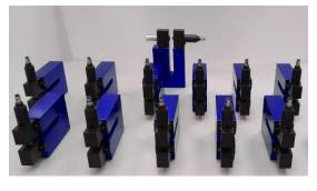
This **HOLE PNEUMATIC PUNCHING MACHINE** is a device that occupies little space and is designed to punch holes in the outer edge of the **MOVING FILM** and in particular, it works with **PLAIN OR PRINTED FILM**. This PU model has to be integrated into **EXISTING MACHINERY** such as extruders, slitters, bag machines, printing machines or any other film
